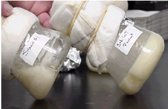
Figures 3 and 4 - Fat Degradation capabilities of two isolates compared to a commercially available grease trap product
